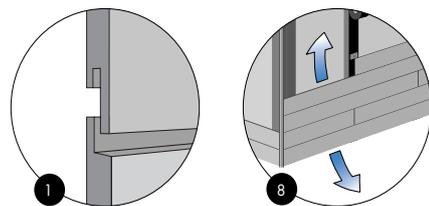
The system includes an air cavity in front of the load-bearing wall, allowing an airflow that prevents heat or moisture accumulation.
